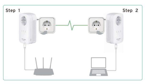
Note: Powerline adapters should be deployed on the same circuit and in set of two or more. The first, connected to the router and others located elsewhere to enable connectivity in those locations.
