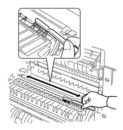
5 While rotating the transfer roller with the gear on its left, move the cleaning brush back and forth along the transfer roller to remove soiling as shown. After cleaning, return the cleaning brush to its storage space, and close the left cover 1 and the front cover.
