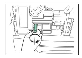
6 Open left cover 1 to remove paper jammed in the MP transport tray.
