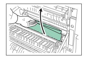
**3** Push the lever (gray colored) to raise the duplex unit and remove the jammed paper.
