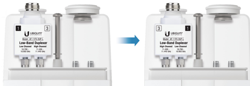
Reversible Duplexers For Easy Channel Configuration
